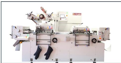
hot foil stamping unit, flat bed die cut unit
