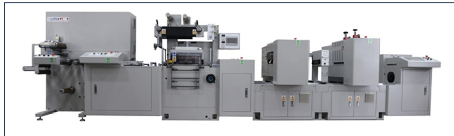
hot foil stamping unit, flexo varnishing unit, semirotary die cutting unit
