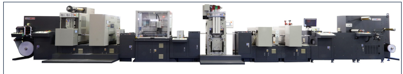
semirotary hot foil, semirotary offset printing unit, screen printing unit, flat bed hot foil unit, flexo varnishing unit, semirotary die cut unit
