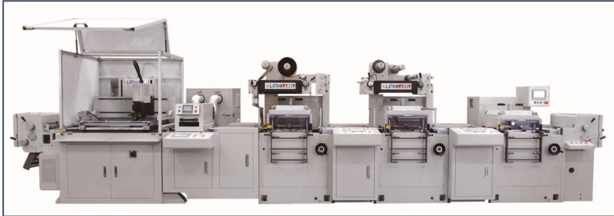
screen printing unit, 2 x hot foil stamping unit, flat bed die cut unit
