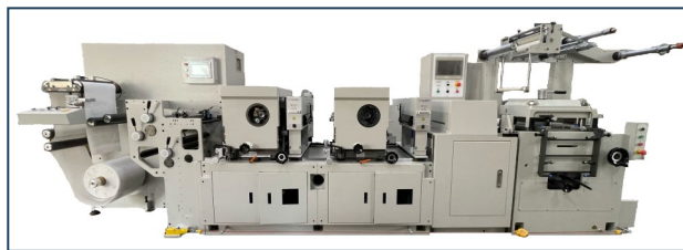
2 semirotary flexo printing units, flat bed die cut unit, lamination unit
